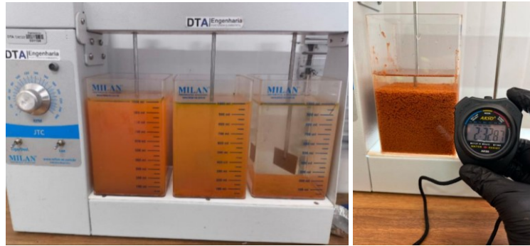
Figure 8. Use of Jar test to determine dosage and flocculation stability.
