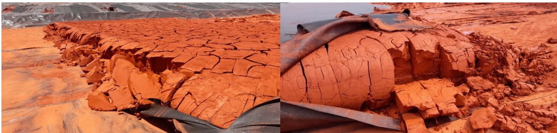
Figure 12. Final condition of the dewatered Geobag.
